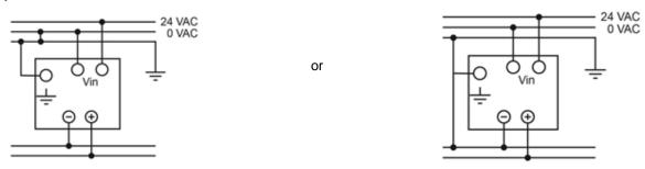
**Output:** Output voltage 24 VDC is made via the positive (+) and negative (-) terminals. The red LED DC signalises the correct output power. When the red LED is blinking, the device is in overload range or in short circuit protection.
