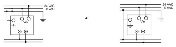
**Output:** Output voltage 24 VDC is made via the positive (+) and negative (-) terminals. The red LED DC signalises the correct output power. When the red LED is blinking, the device is in overload range or in short circuit protection.
