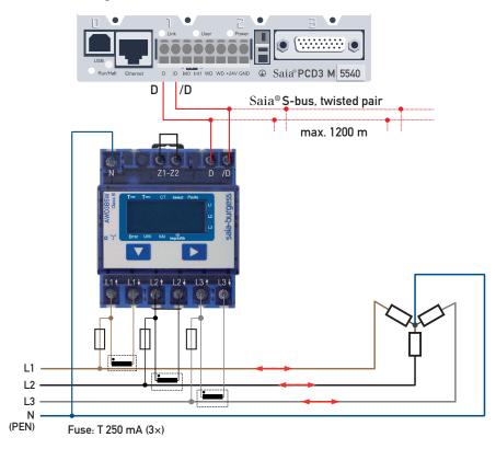
The secondary connection for the current converter on the network side is connected to the measuring phase. The current converter may not be earthed for this reason.
